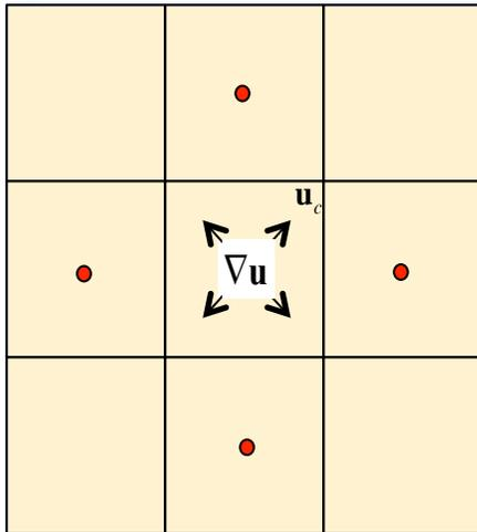
3<sup>rd</sup> order uses a 9-point stencil is **more accurate at the corners than 2<sup>nd</sup> order**
