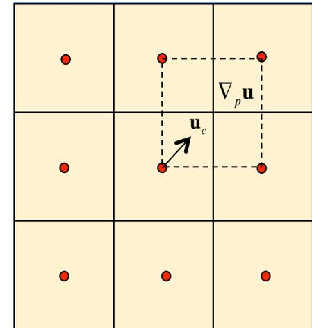
9-point stencils require special handling of ghost cells at mesh corners
