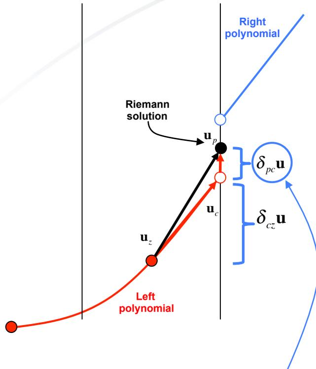
The surface fluxes can be decomposed into a **reconstruction** and a **discontinuity**
