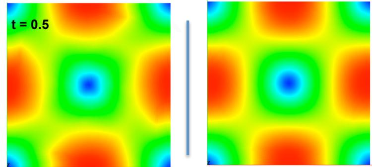
The flow should be incompressible and the velocity field should not change with time
