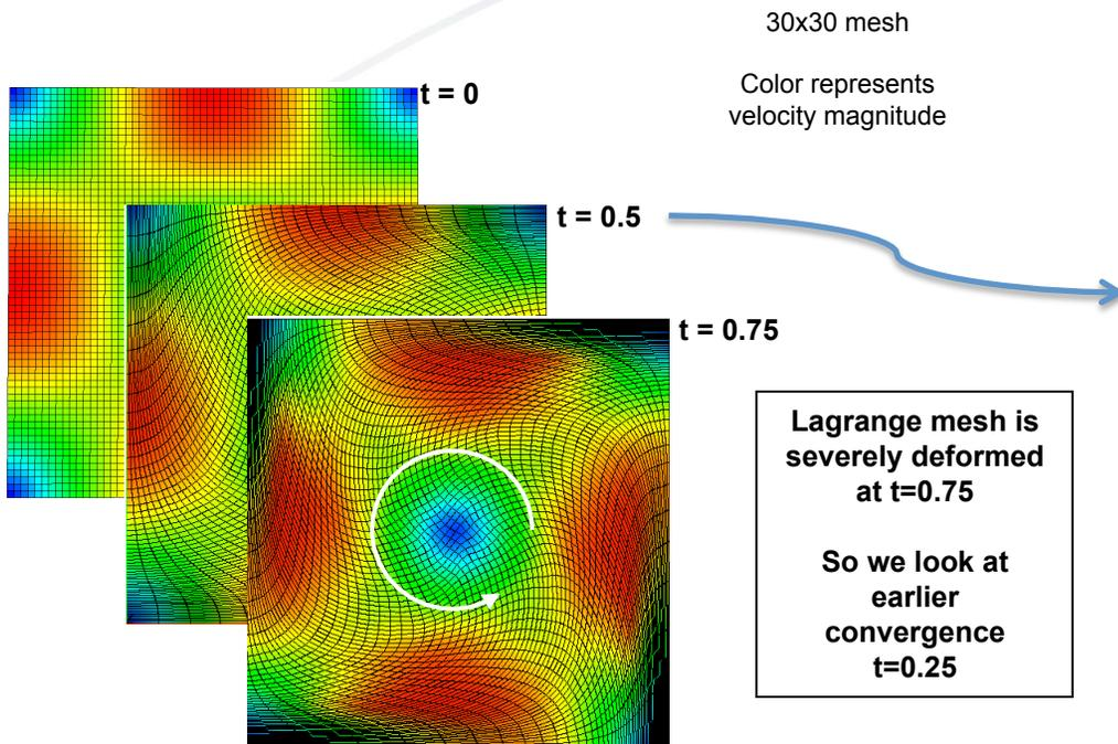
Lagrange mesh is severely deformed at t=0.75
