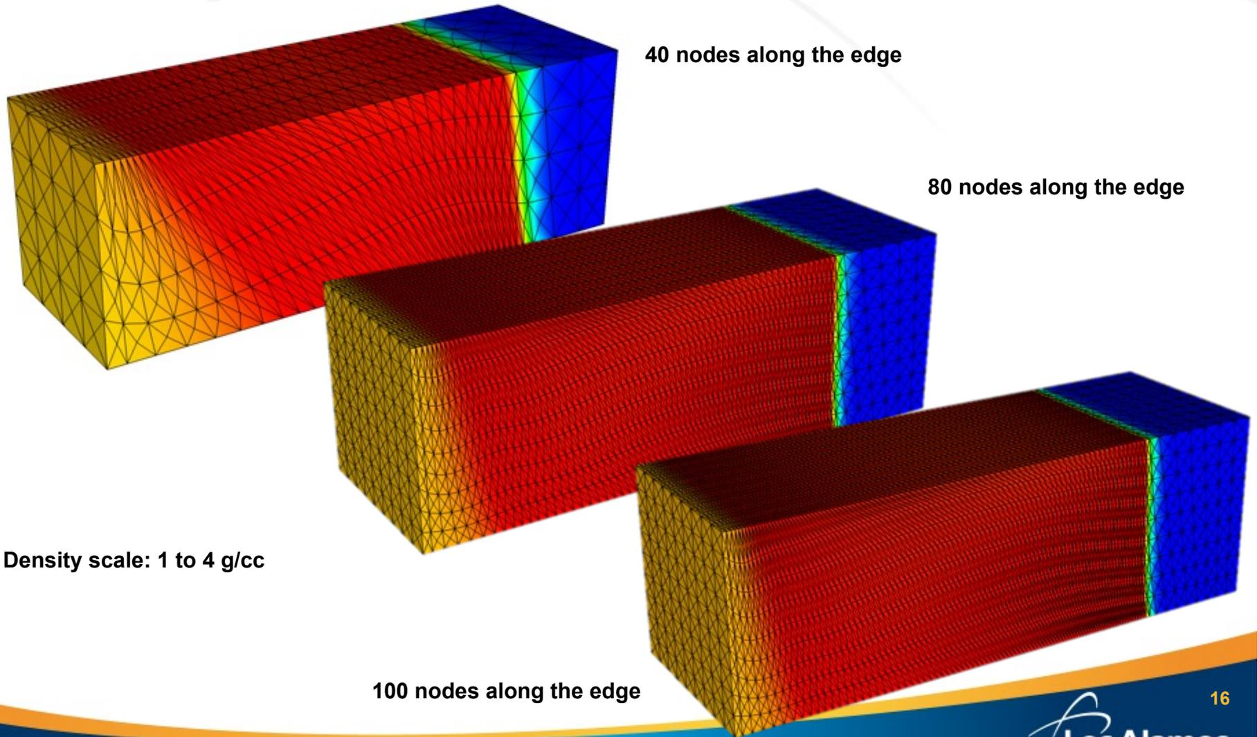
The mesh robustness on Saltzman is maintained after the shock reflects from the wall
