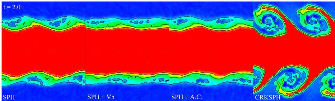
Figure 1: Snapshots at  $t = 2.0 \approx 5\tau_{\text{KH}}$  of the growth of a Kelvin-Helmholtz instability in density for (from left-to-right) traditional SPH, SPH with “grad-h” corrections, SPH with artificial conduction, and CRKSPH.
