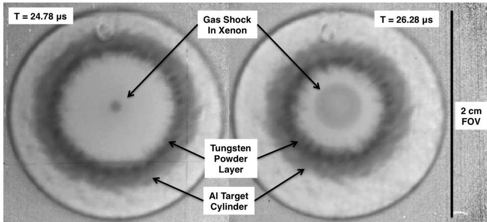
Figure 1: Axial proton radiographs of the DSH-2 experiment at two different times showing the shock in the Xe gas, the tungsten powder layer, and the Al target cylinder.
