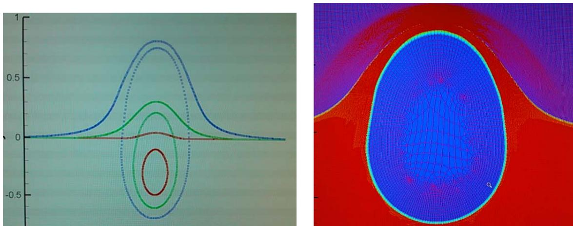
Figure 1: Numerical results of underwater explosive problem computed by new ALE method. Left: Evolution of material interface, right, the computational grid near the material interface.
